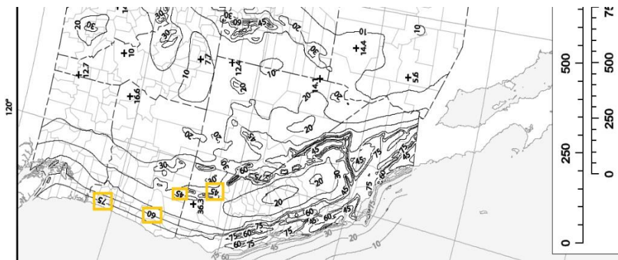
Figure 22-2 Uniform-hazard (2% in 50-Year) ground motions of 1.0-second spectral response Acceleration (5% of critical damping), Site Class B
